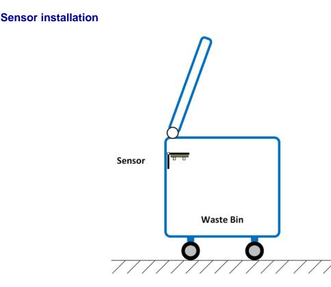
To install the sensor use four (4) 5mm screws with nut to secure it safely on the back of the waste bin.
